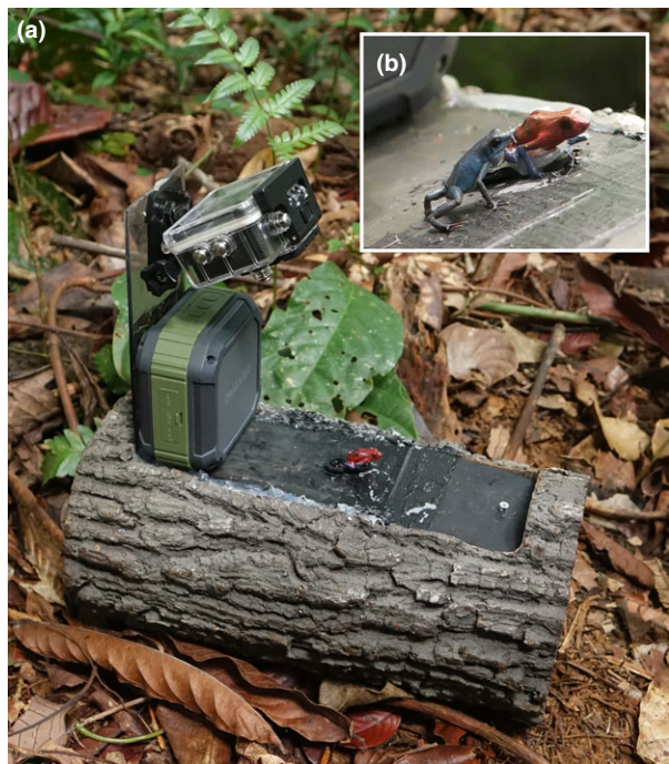
Fig. 2 Experimental setup used in stimulated intrusion trials to quantify male aggression towards red- and blue-coloured opponents. (a) Hand-painted plastic models were mounted onto a radio-controlled servomotor hidden in a log-shaped cylinder. Advertisement calls were played through a Bluetooth speaker located behind the model. (b) Photograph of a blue territorial male attacking a red frog model during a trial. See also Video S1.
